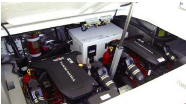
On this express cruiser a large cockpit section lifts electrically offering good access. Electric lifts should have a manual release in case the power fails, but they're often heavy to open.
