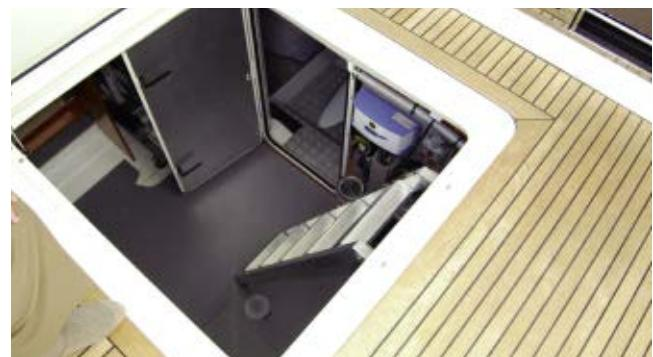
This is the entrance to a very spacious and well-rigged engine room, but it's six steps down the ladder and as you're trying to get your footing, there's not much to hang onto. Gas lift struts hold the hatch cover open.
