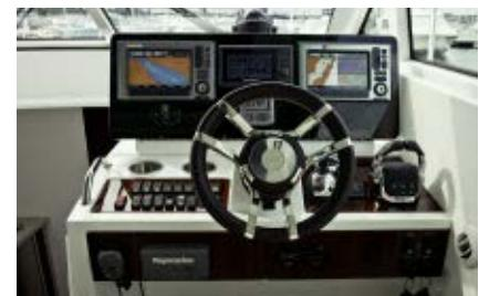
The helm is one of the very best features on the 41 Cantius. It's neatly laid out and the ergonomics are very good, but the unique feature is that the dashboard is cut out ahead of the instrument binnacle, flooding the lower deck with natural daylight.
