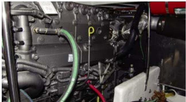
To maximize the interior accommodations, this yacht has the floor down as close as possible to the top of the diesel engines. The area is really too small for an owner to safely get in unless they lift out the floor panels over the engines.
