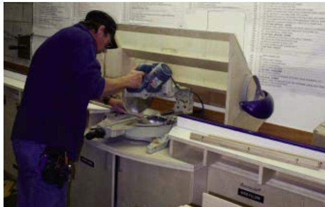
In the woodworking shop, a part is trimmed on the chop-saw. A master list of all wood components is displayed on the shop wall behind the saw.
