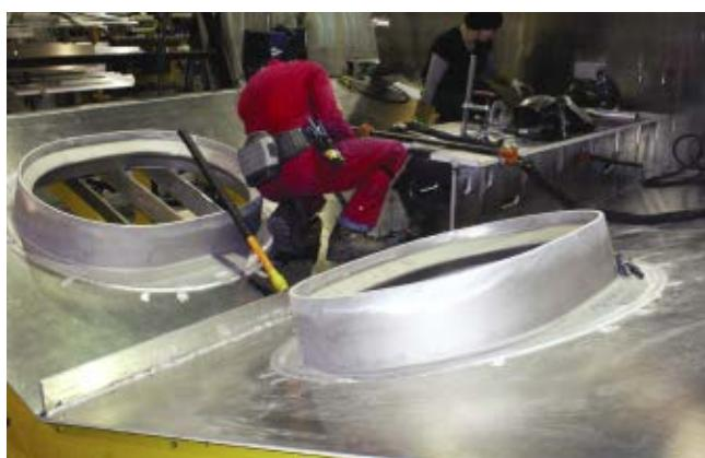
Looking forward into the engine room of a new 56-footer with mounts for the IPS drives newly welded in place and the central bench of the engine room receiving final installation welds.
