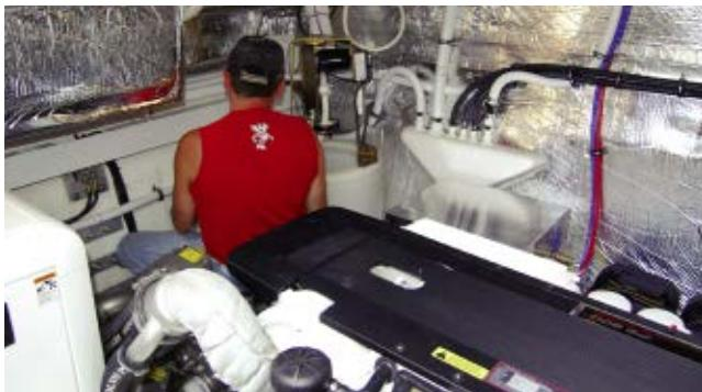
This is the engine room on Cruisers Yachts 48 Cantius looking over the port side Volvo IPS diesel engine to the transom where a technician is working. The lighting is very effective and there is 50 inches of headroom.
