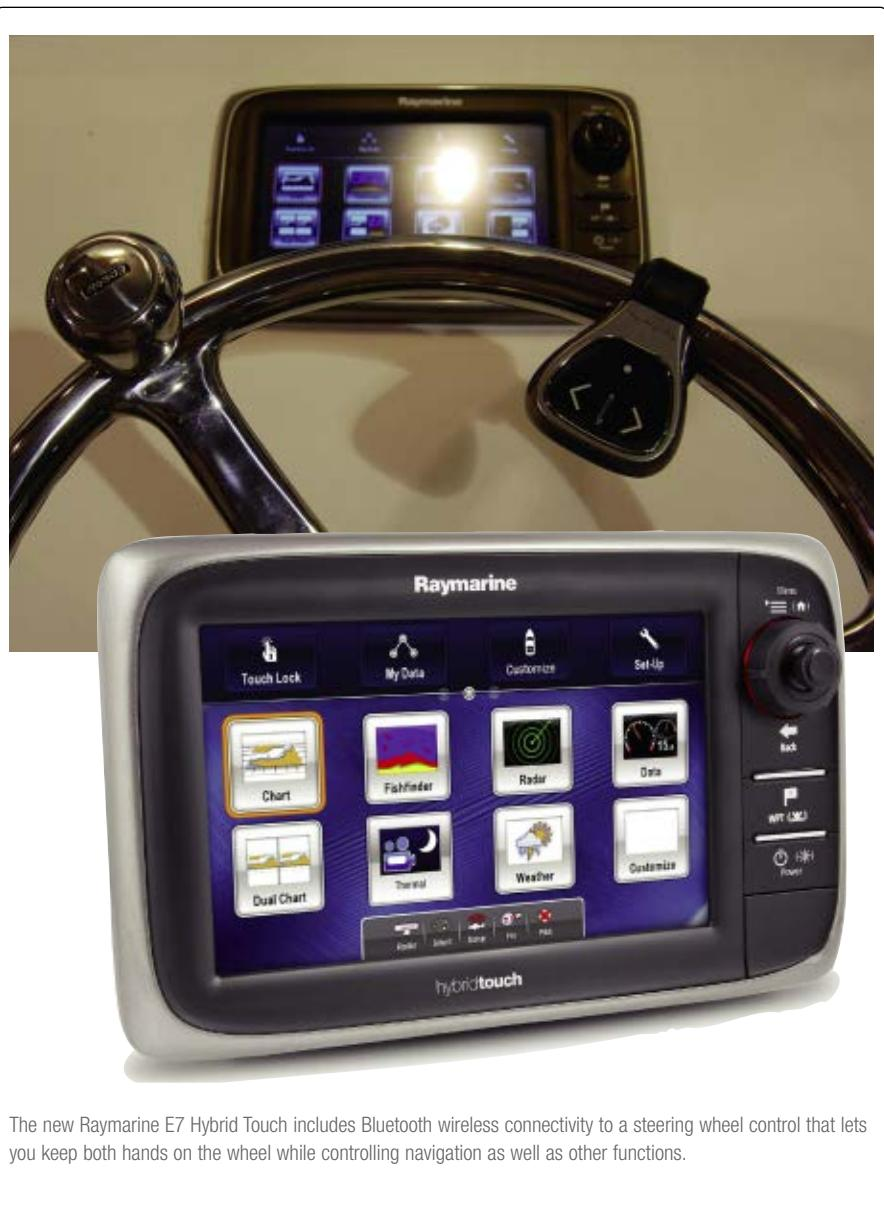
The new Raymarine E7 Hybrid Touch includes Bluetooth wireless connectivity to a steering wheel control that lets you keep both hands on the wheel while controlling navigation as well as other functions.
