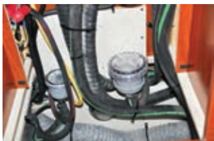
➤ Ensure that the raw water strainers are clean, clear and that the caps are put on securely to prevent vacuum or water leaks.
